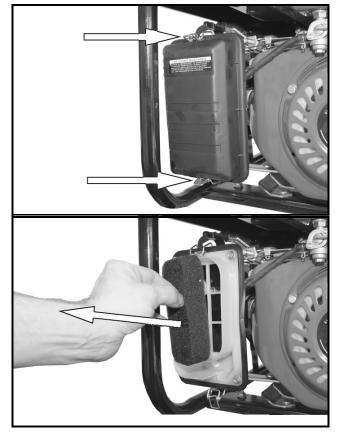
dry completely, once it is dry immerse in clean engine oil and squeeze to remove excess oil.
